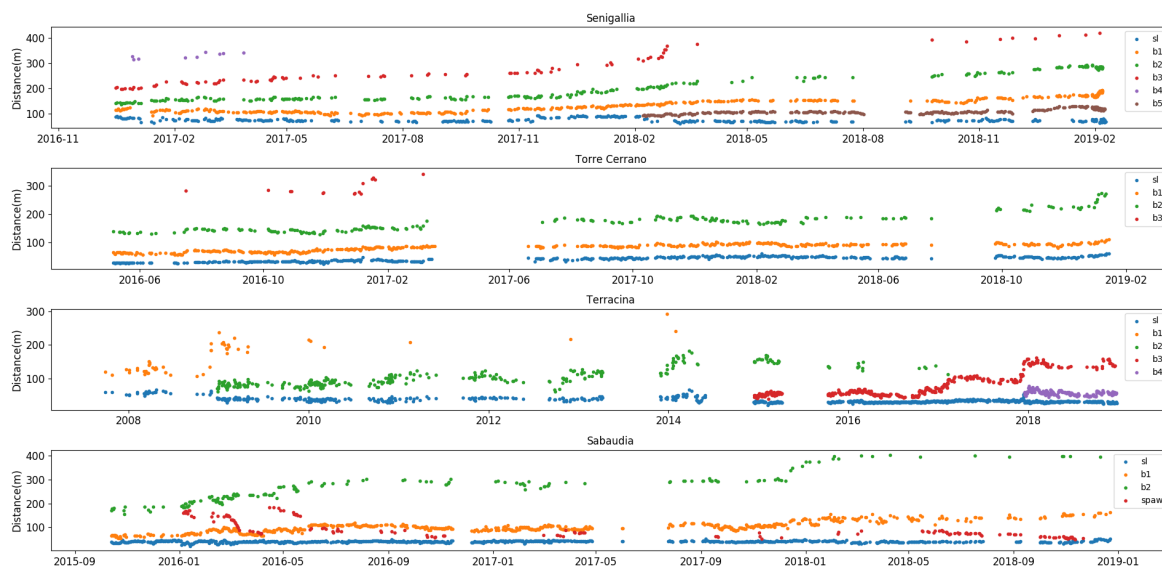
Figure 4. Time evolution of locations of shoreline and barlines in Senigallia, Torre del Cerrano, Terracina and Sabaudia. Each dot represents the daily-averaged location of the relative beach feature.
